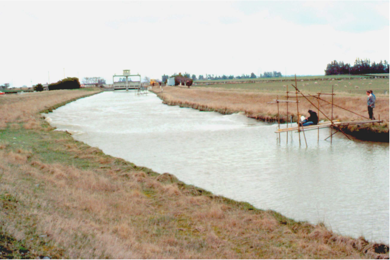
Photograph 1: Surge Tests on the Rangitata Diversion Race
